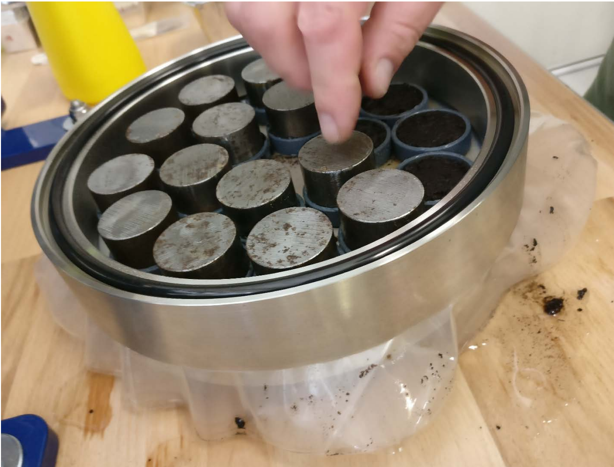
Figure 2 Placing the weights on top of the sample cylinders in the press.
