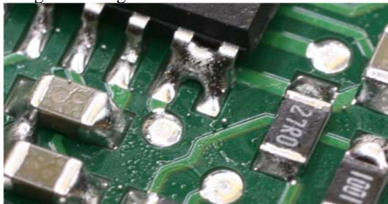
Figure 5. Solder bridge between the last 2 legs of an IC.
