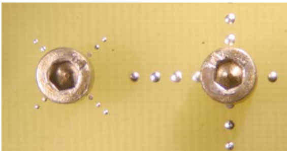
Figure 6. Two types of bolt head patterns. Two solders are missing.
