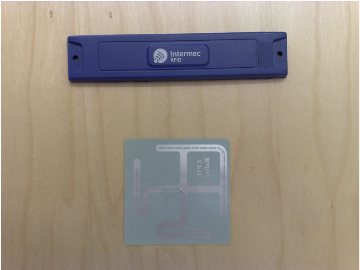
Figure 34: Tag sample No.1: a stick-like UHF tag (above). Tag sample No.2: a slice-like UHF tag (below).
