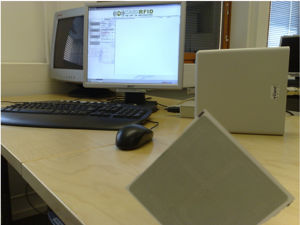
Figure 40: tag No. 2 work well in front of the reader antenna
