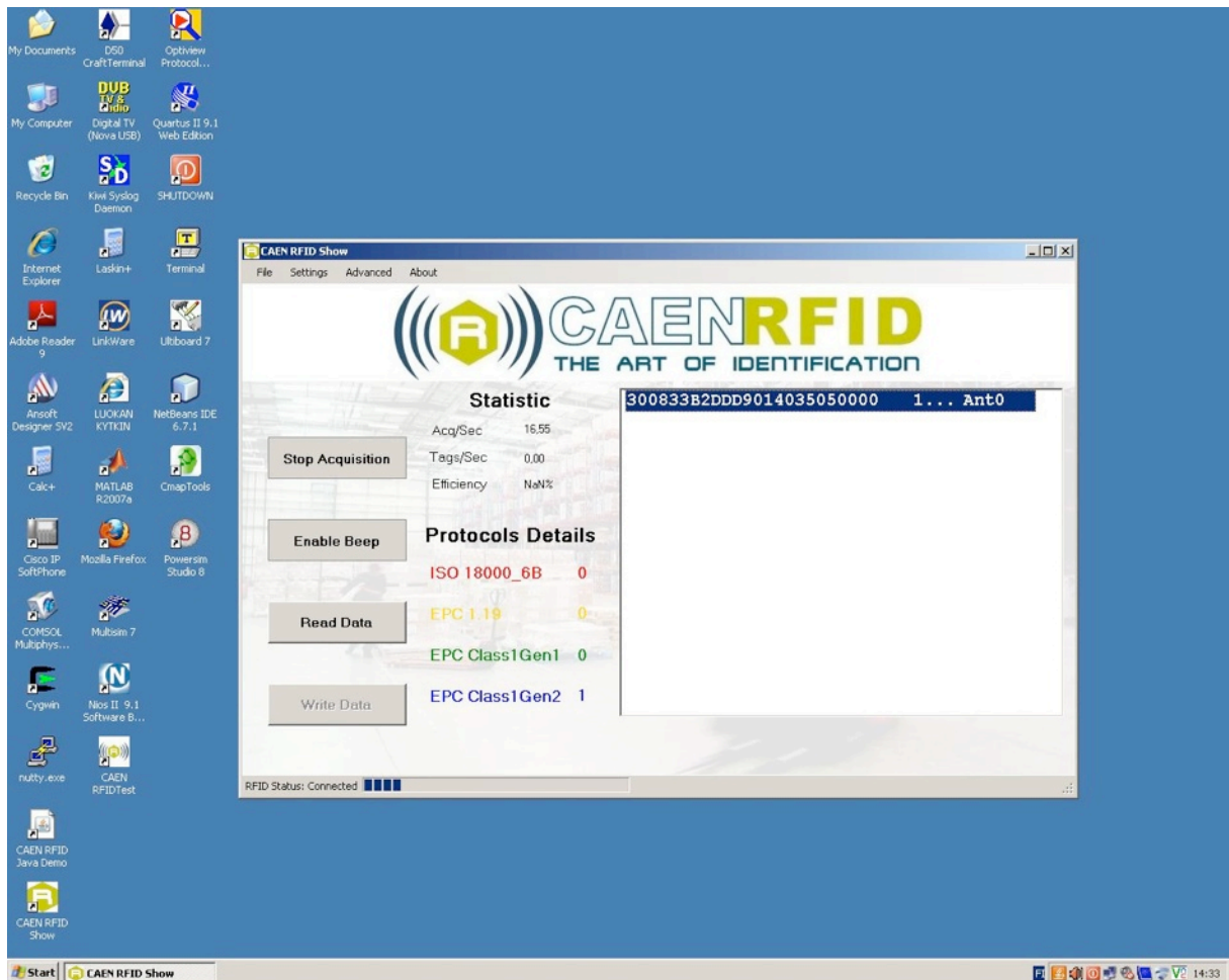
Figure 38: CAEN RFID Show successfully detect a EPC Class1 Gen2 tag
