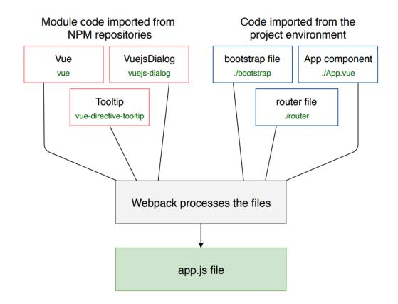
Figure 4. Illustration of Webpack operation logic.
