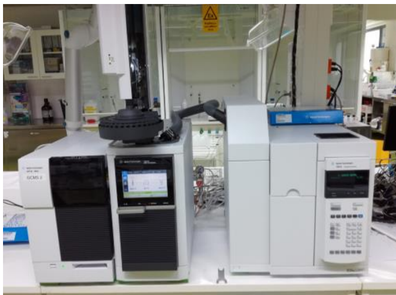
FIGURE 9. The MSD and GC are to the left, installation to the right is the headspace-installation simultaneously connected to the gas chromatograph
