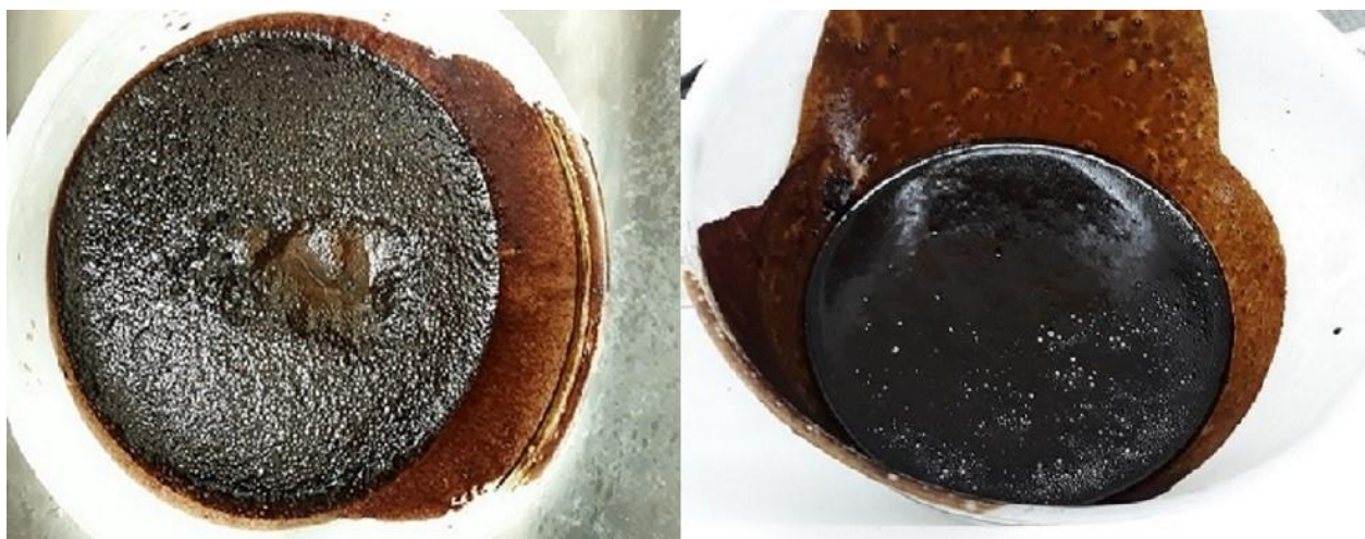
Figure 35. A visual comparison between reference adhesive without additives (left) and adhesive + defoamer 2 (right). The pictures were taken after 3h settling time.
