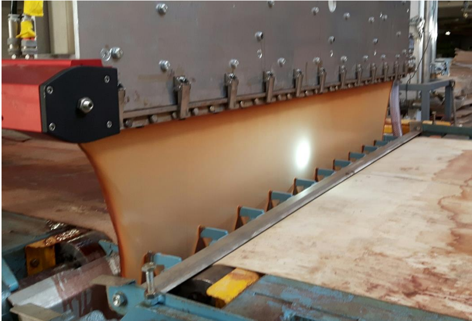
Figure 3. Basic curtain coater with a pressure head. (UPM, 2018)
