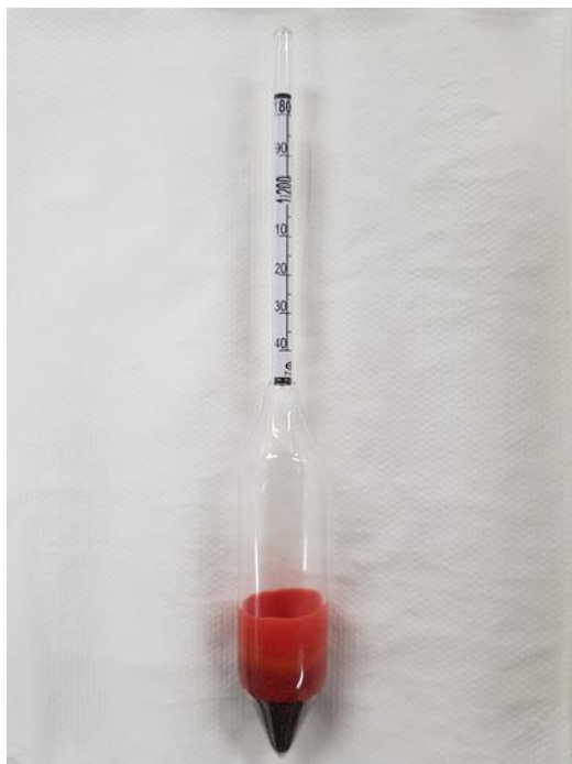
Figure 23. Areometer for measuring relative density of liquids.
