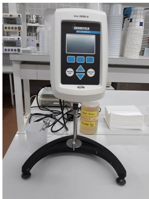
Figure 19. Brookfield DV1 viscometer with a 02-spindle attached.
