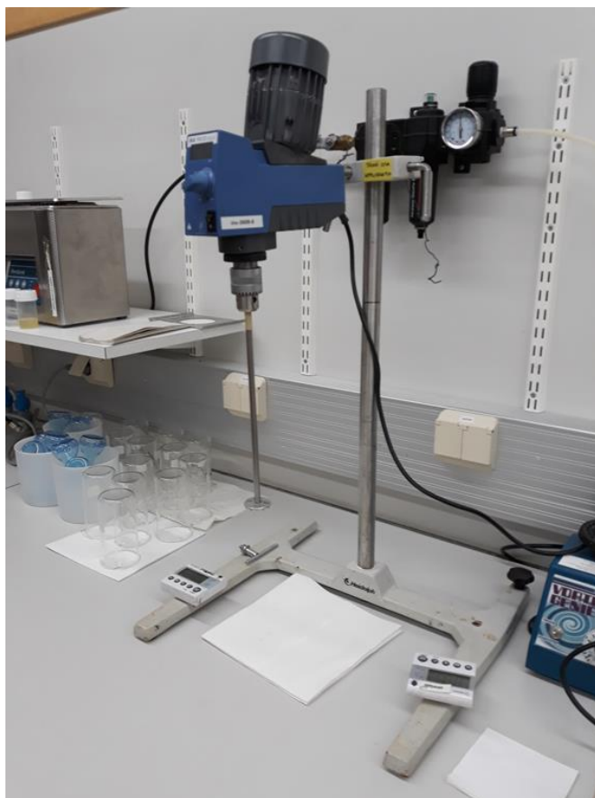
Figure 21. The laboratory stirrer used for conducting the stirring tests.
