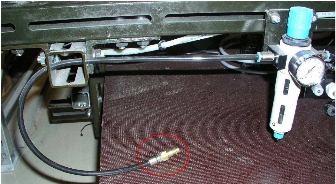
Image 5. Pressurised air feed connector (circled in red).
