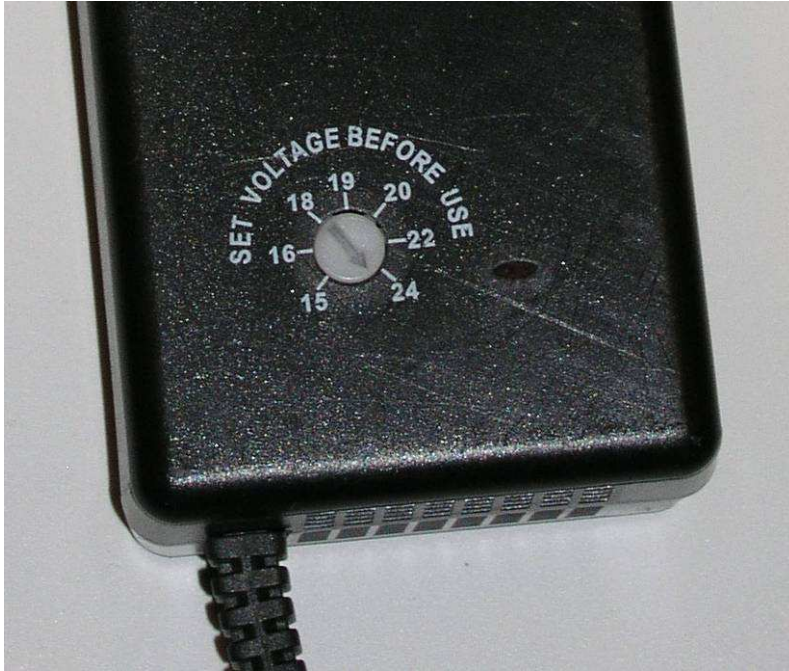
Image 3. Voltage selector on the power source
