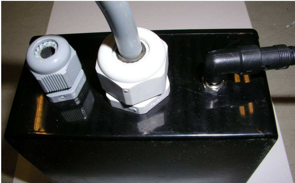
Image 4. Power source connected to remote controller. Connector on the right.
