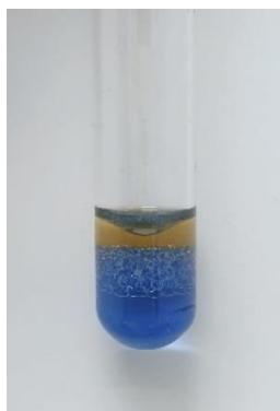
PICTURE 7. Emulsion formation when using chloroform to extract indigo
