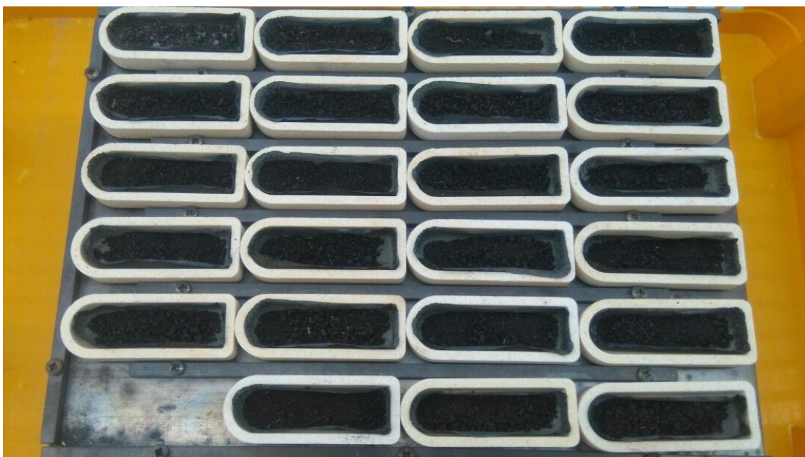
PICTURE 5 Samples in ceramic dishes before being calcined in muffle furnace
