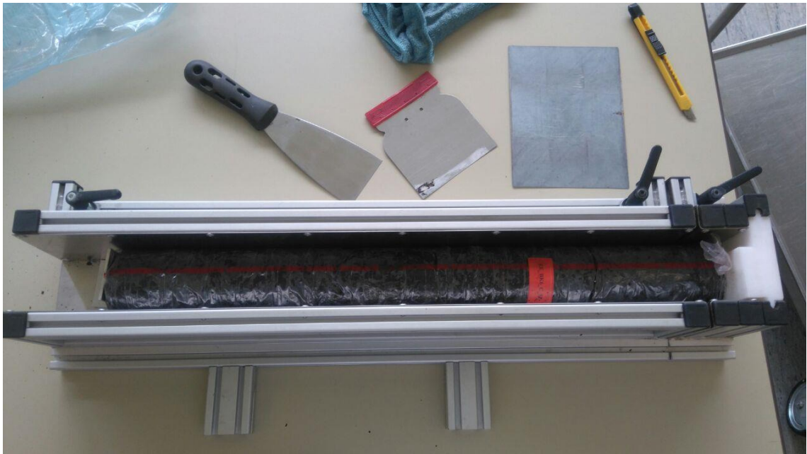
PICTURE 2 Cutting soil core in the laboratory
