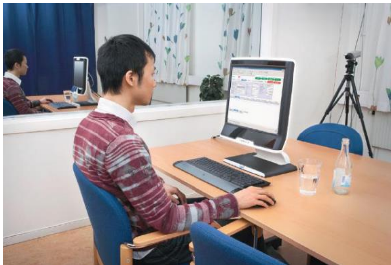
Figure 10: A screen-based Tobii Technologies eye-tracking device in use (Bergström, J.R. & Schall, A. 2014 p.4)
