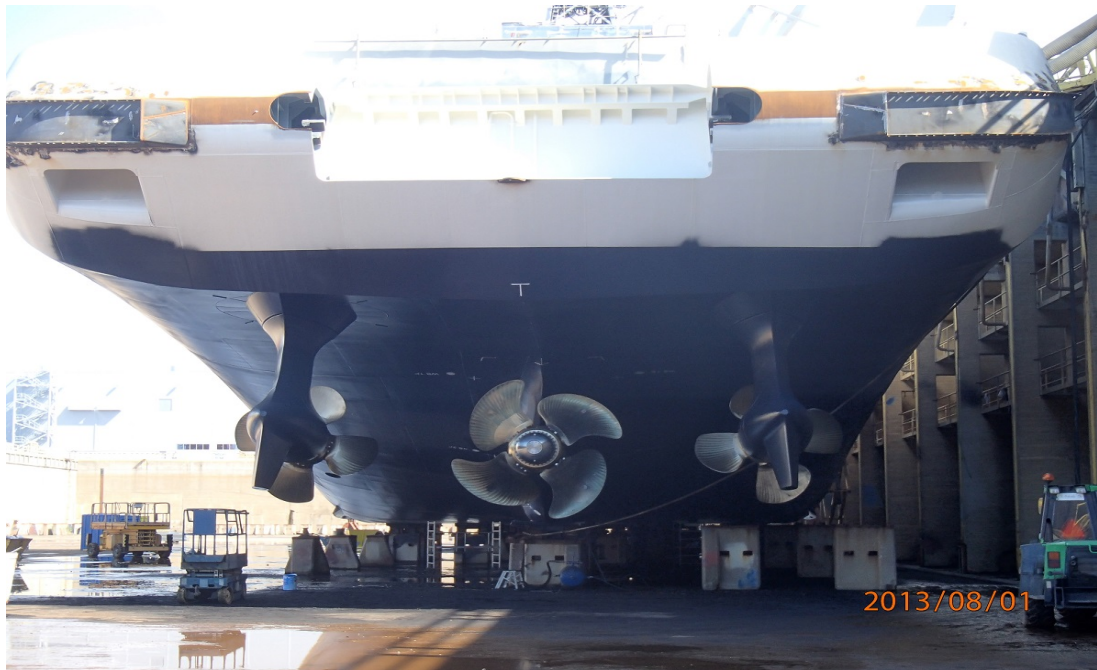
Picture 32. Finnish border guard vessel Turva hybrid propeller arrangement with two CPP azipulls and one conventional shaft with CPP propeller. (Saarinen, 2013)
