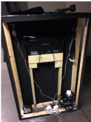
PICTURE 14. The electronics inside of the 'electronics hull'. This part was not visible to gallery visitors, as it was later closed off with another board.
