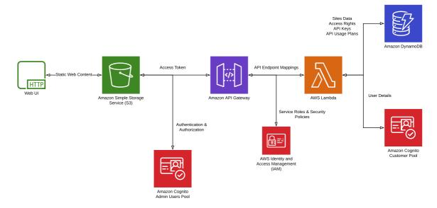
Figure 1. Overall Application Architecture
