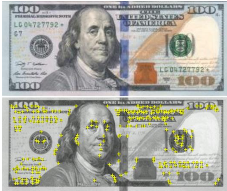
Figure 1. Example of how Vuforia Engine tracks an image (PTC Inc. 2018a.)
