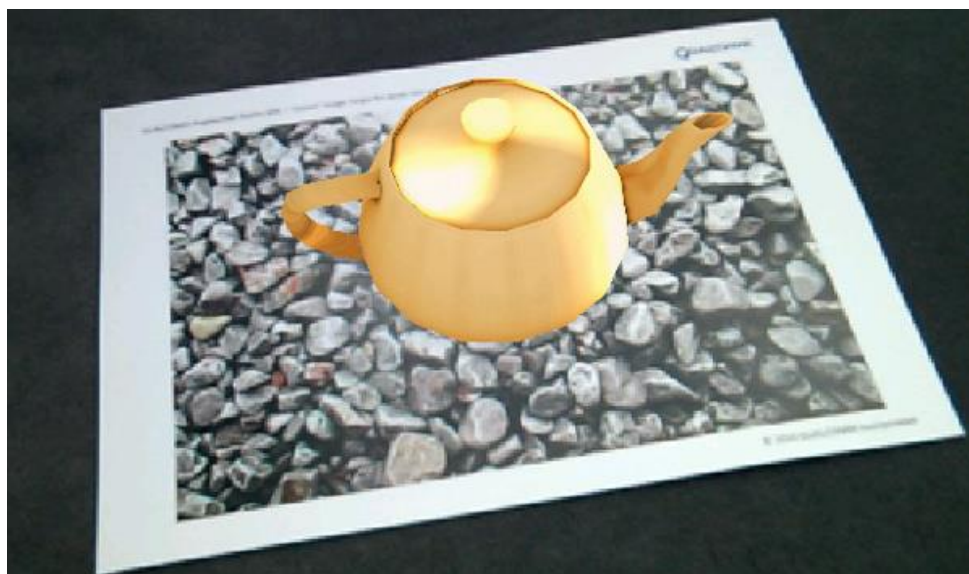
Figure 2. A teacup augmented onto an image target of rocks (PTC Inc. 2018a.)
