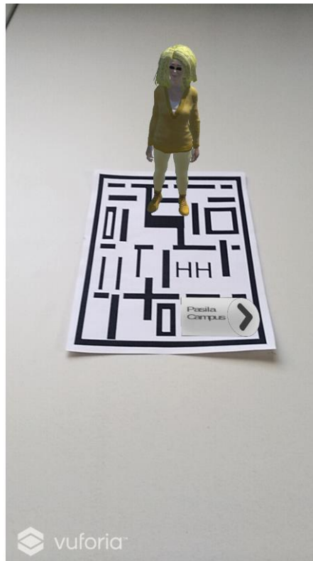
Figure 11. 3D model augmented onto image target with a virtual button on the lower right
