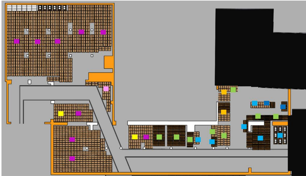
Figure 40. Location of goods based on colour zones in “Spritzerei” warehouse (ground floor)
