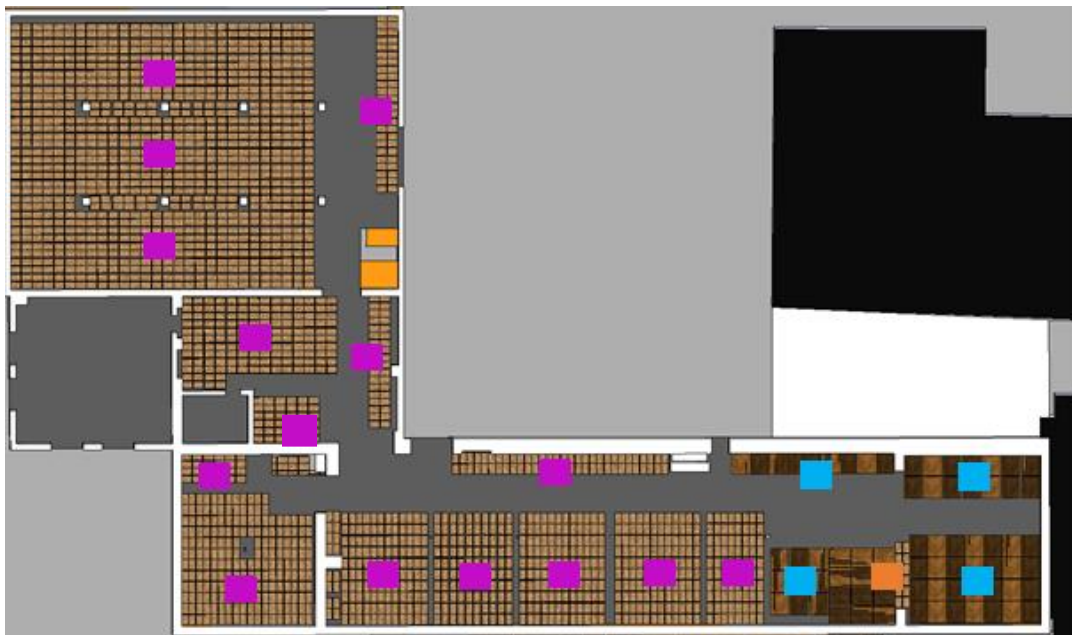
Figure 41. Location of goods based on colour zones in “Spritzerei” warehouse (first floor)
