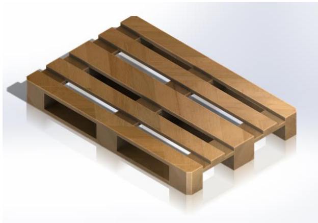
Figure 5. 3D model of a stamped euro size pallet (1200 x 800 mm)
