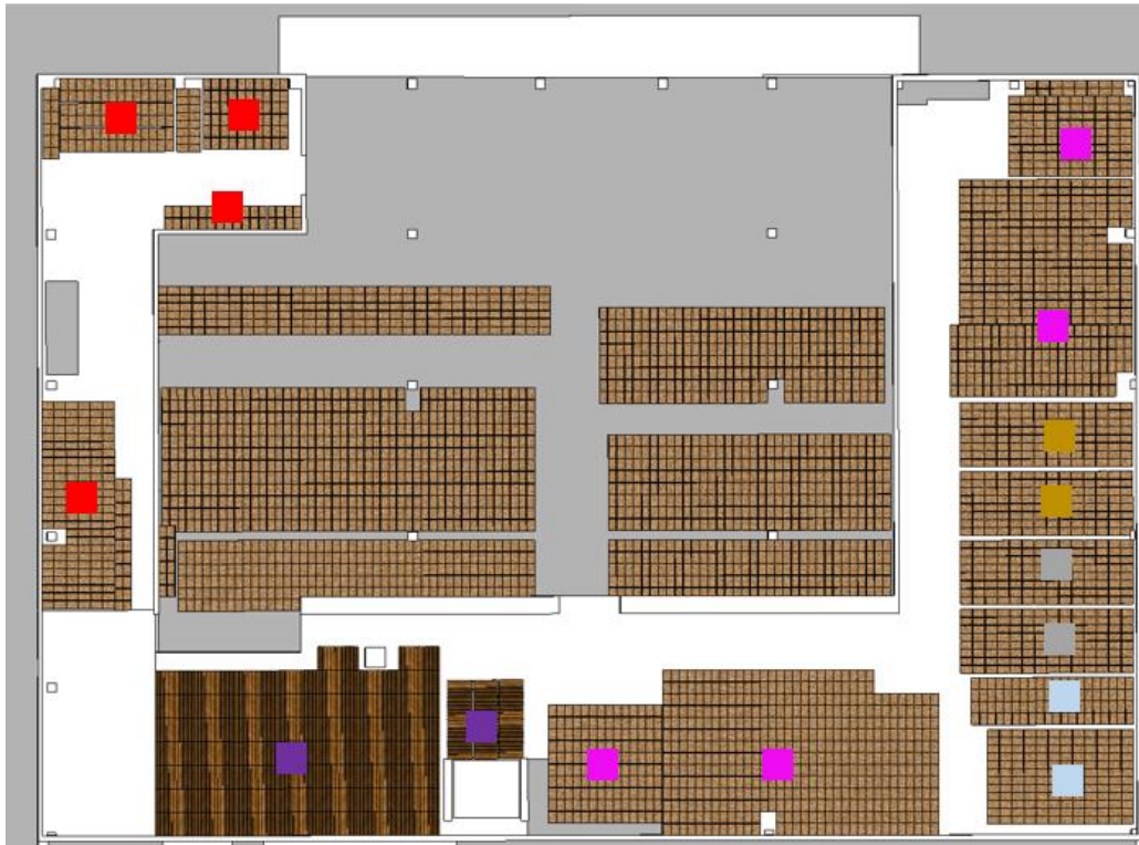
Figure 38. Location of goods based on colour zones in “Blaserei” warehouse (mezzanine floor)
