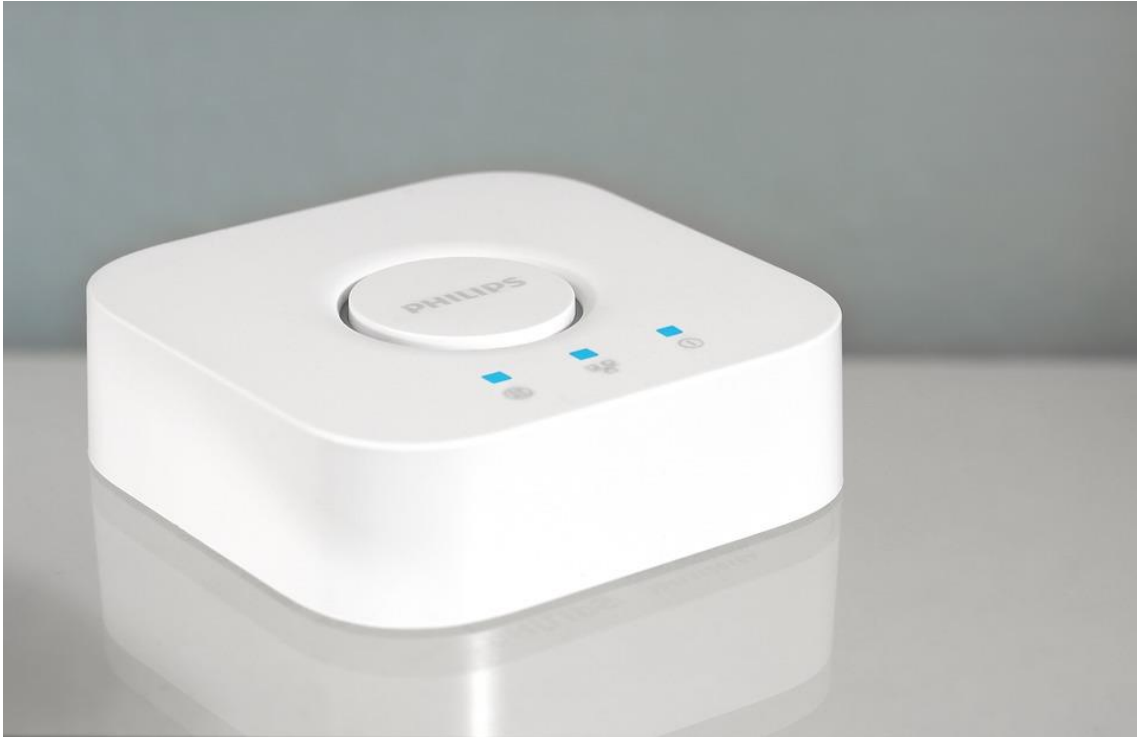
FIGURE 4. Philips Hue Bridge [6]
