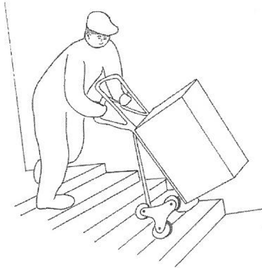
Figure 5.5 Stair handcart (Raturva 2, p. 27)
