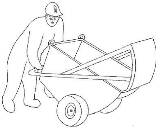
Figure 5.6 Tip-over handcart (Raturva 2, p. 27)
