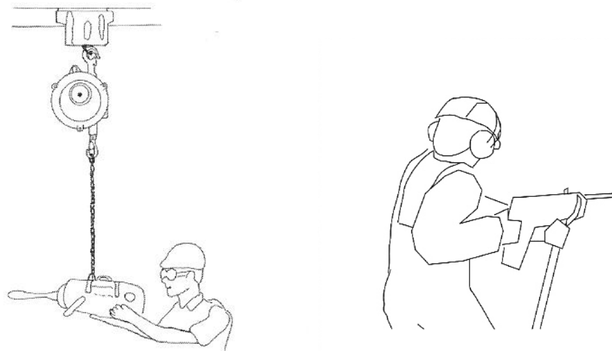
Figure 5.13 Support for a drill or screwdriver and a device for lightening the load (Raturva 2, p. 28)
