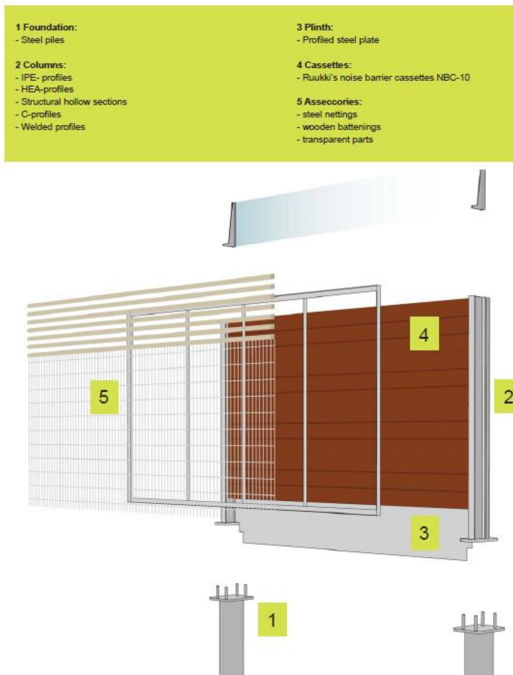
Figure 2.1 The basic structure of Ruukki's noise barrier structure (a misprint in illustration: NBC-95 instead of NBC-10)
