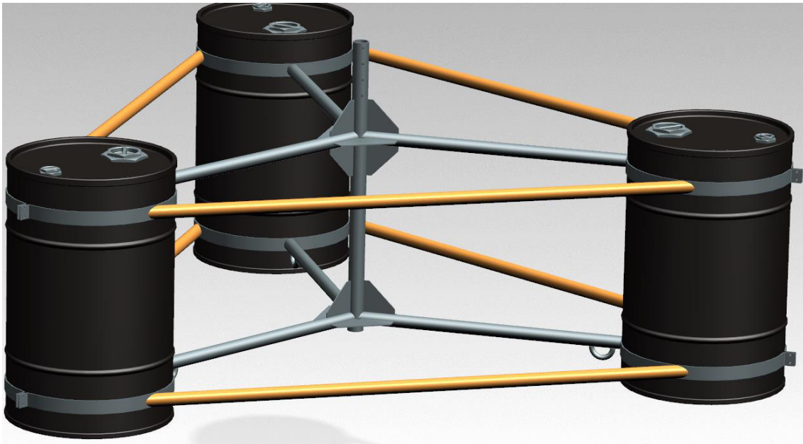
Figure 17: Perimetral support tubes
