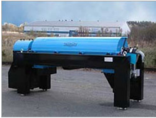
(Sludge Dewatering: Noxon Decanter Centrifuges )
