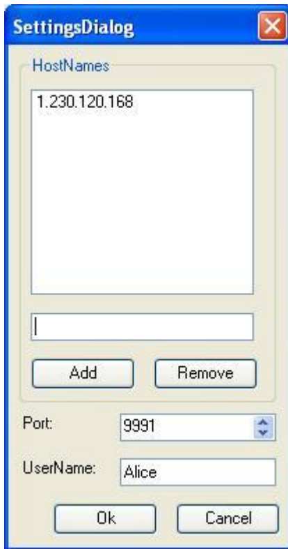
Figure 19. Settings from a P2P chat application showing that the communication is based on a LSI address.
