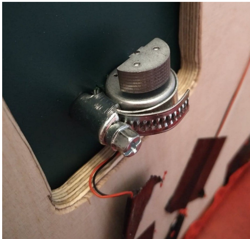
Figure 12. Installation of the vibration motor (Hakkarainen, 2019)
