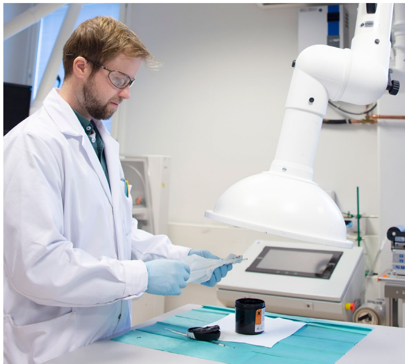
Figure 39. A laboratory environment with a local exhaust systems. Photo credit: Anne Peltola.
