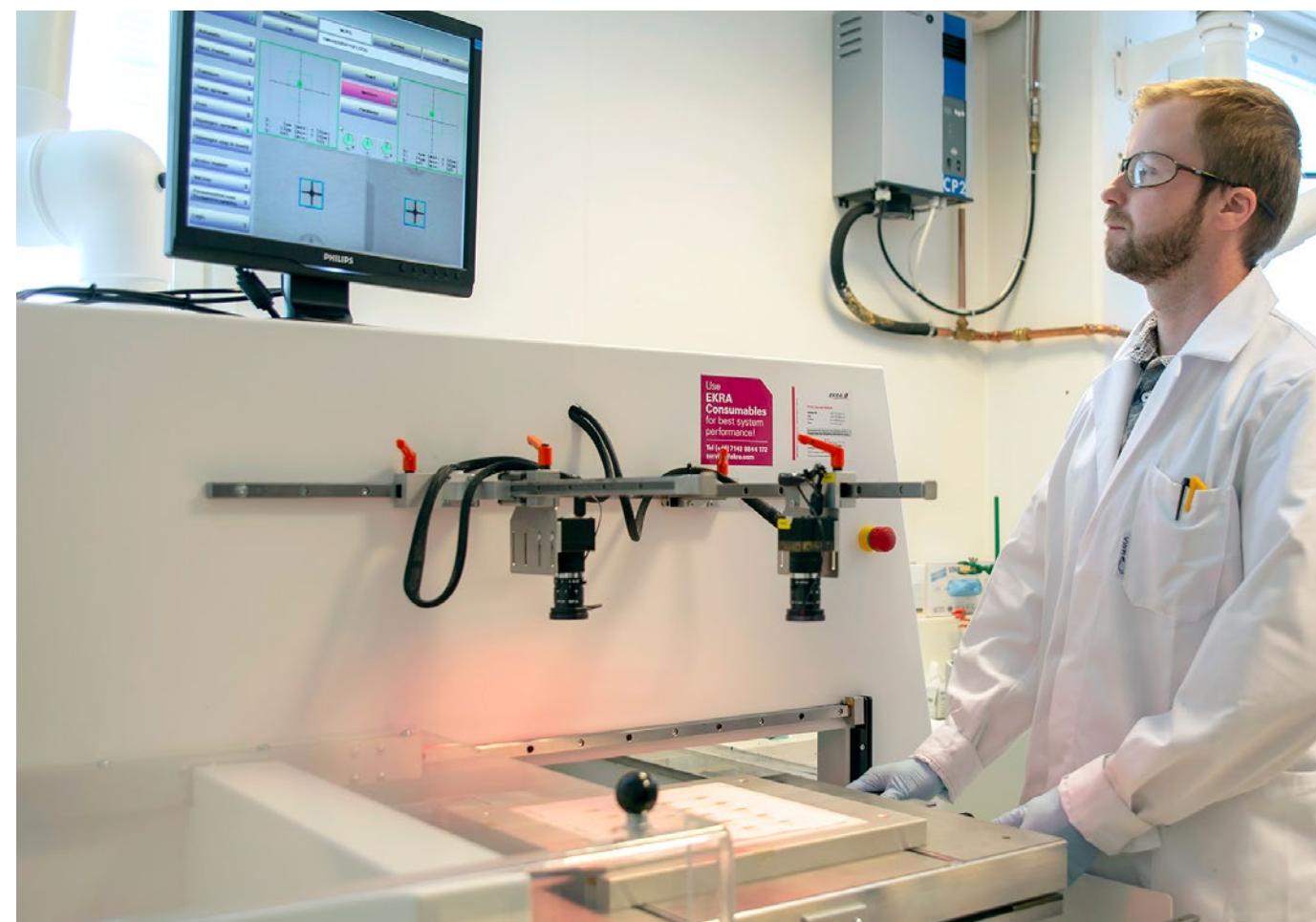
Figure 2. Screen printing with an EKRA E2 printer. Photo credit: Anne Peltola, Design Inspis Oy.
