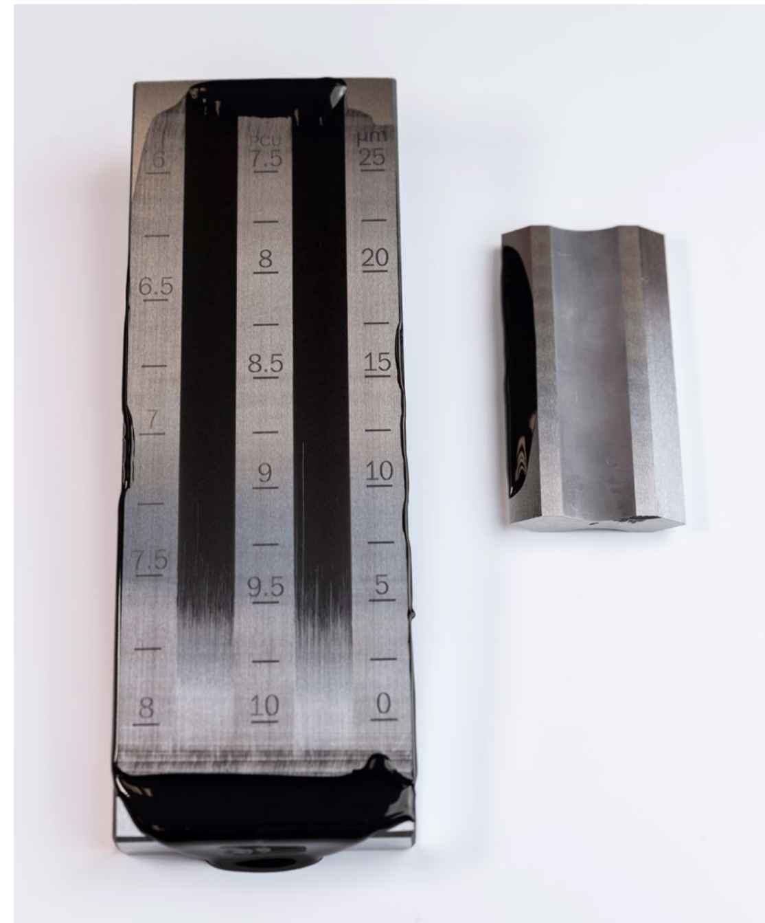
Figure 25. The principle of a grindometer. Photo credit: Jenina Bomström.
