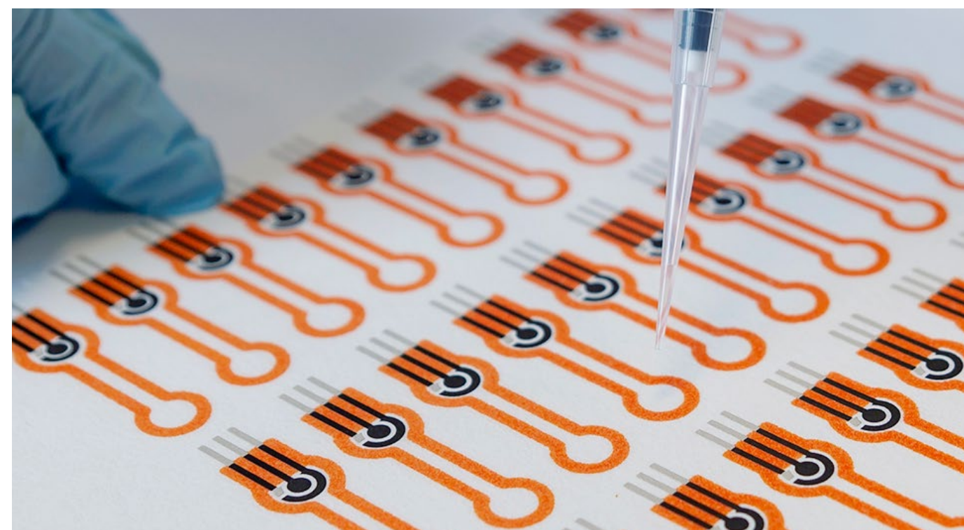
Figure 27. A paper-based biosensor with a fluidic channel printed with carbon, silver and polymer inks. Photo credit: Anne Peltola.
