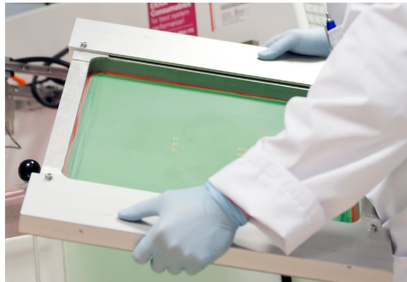
Figure 9. Checking the mesh quality. Photo credit: Jussi Tuokkola.
