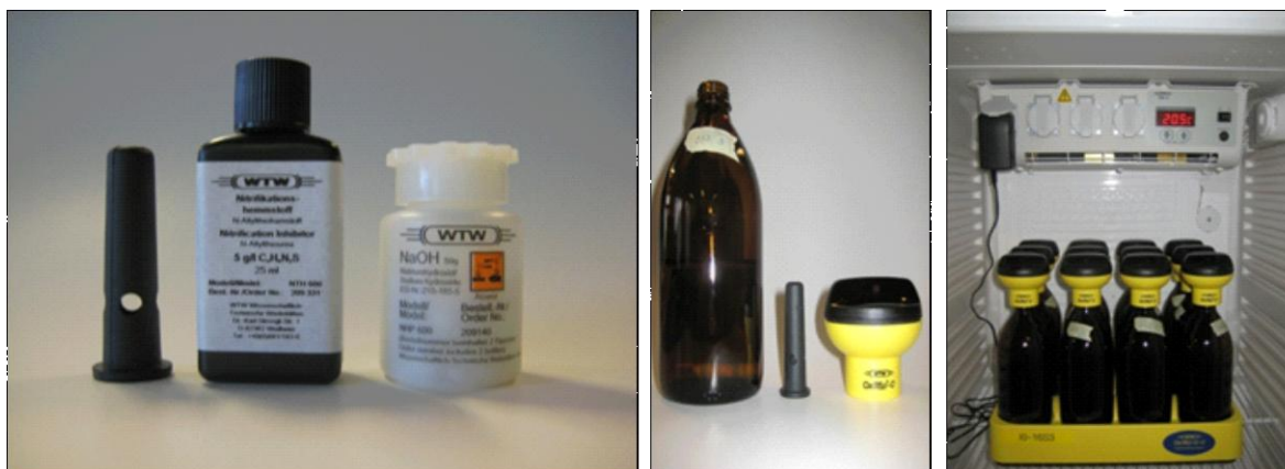
Figure 4 OxiTop measuring system - (left) rubber sleeve as a CO 2 trap, ATU and NaOH pellets, (middle) measuring vessel, rubber sleeve and measuring head, (right) Incubator and magnetic stirrer
