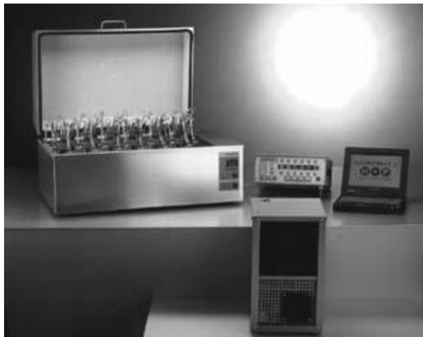
Figure 3 Sapromat ® E measuring system (H+P, 2010) with the water bath and PC measuring unit
