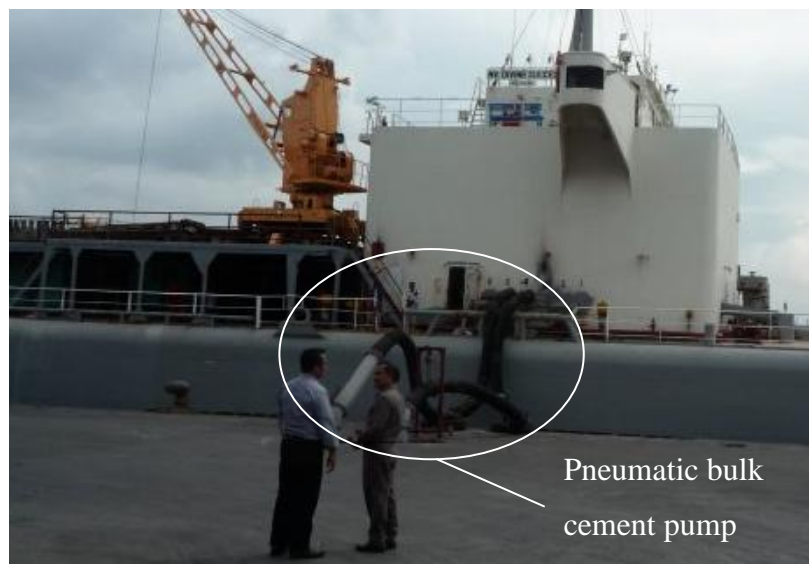
FIGURE 24. Bulk cement loading with pneumatic pump (CEL Consulting, picture library, Indonesia, July 17 2010)
