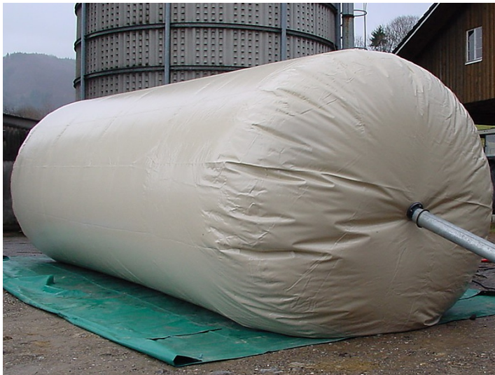
Figure 4: External biogas storage – A gas bag (Novatech GmbH 2011)
