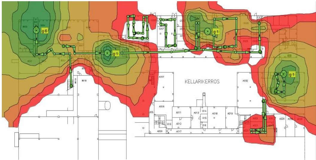
Figure 12. Signal Strength present on the ground floor.
