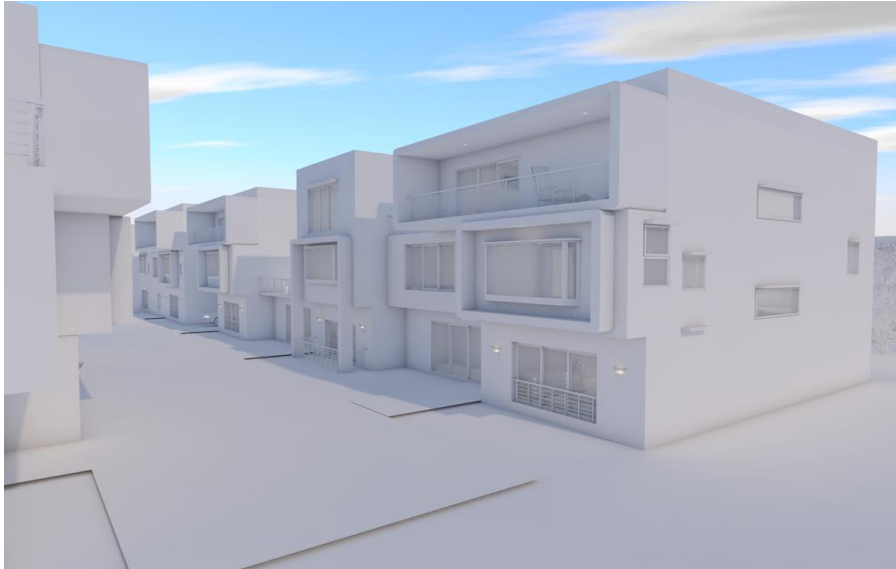
Figure 24. White model render showing passive design techniques like shading, projections, big windows
