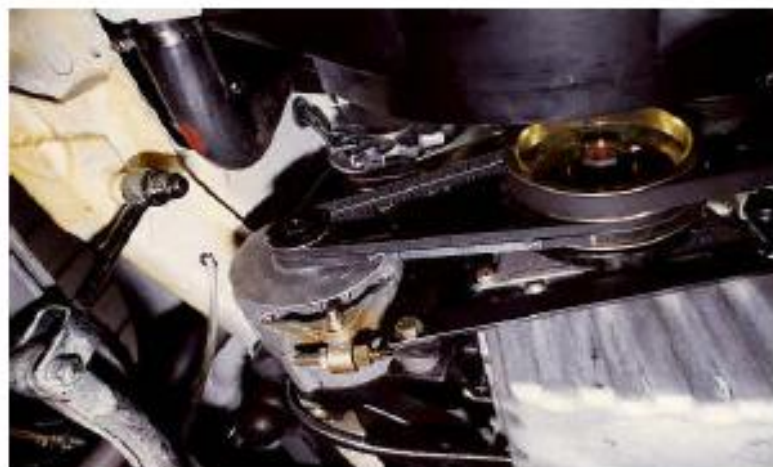
Generator Installation with 2x9,5mm V-Belts
