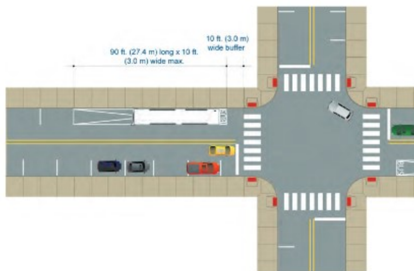
Figure 1: Typical far-side curbside stop configuration
