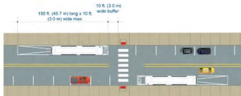
Figure 3: Typical midblock curbside stop configuration
