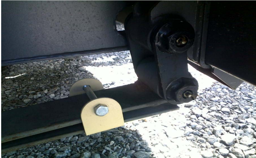
Figure 2. Spring with the clamp installed. (Normet Group, Marketing databank)
