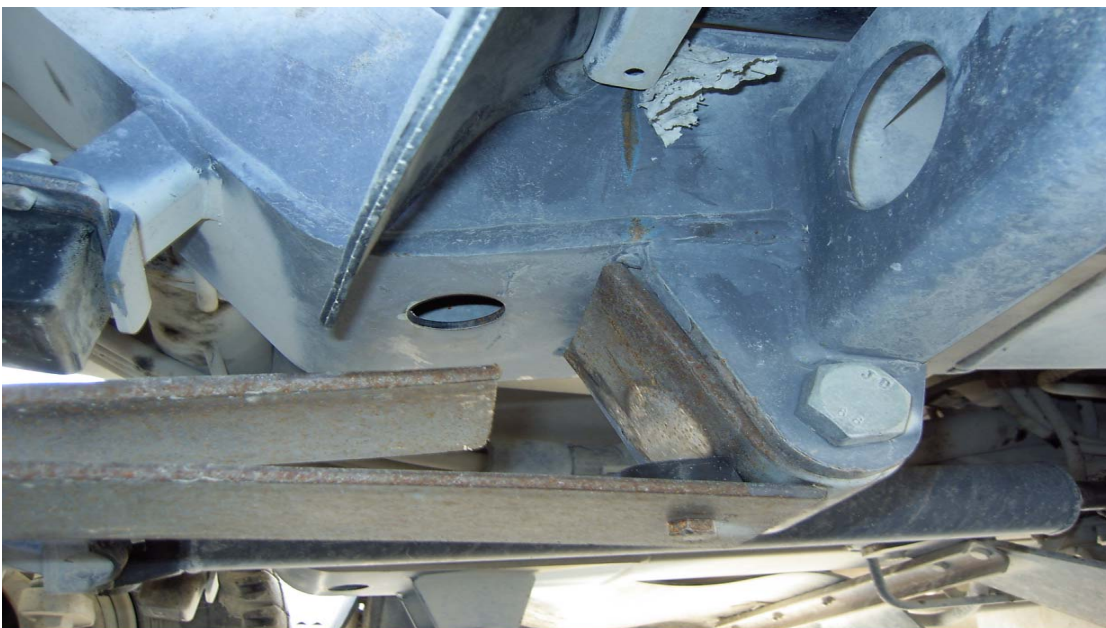
Figure 1. Broken spring in the front axle. (Normet Group)
