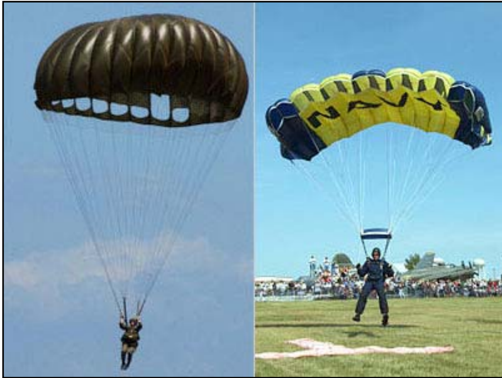
Picture 4. U.S. Army old round canopy (left) and Navy new ram-air canopy (right) [22]
