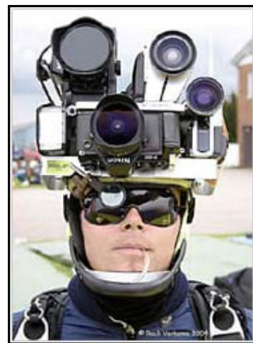
Picture 9. Ahti Kangas wearing a complex multiple camera helmet setup with a sight and a pressure switch. © Rauli Verkamo. [5]
