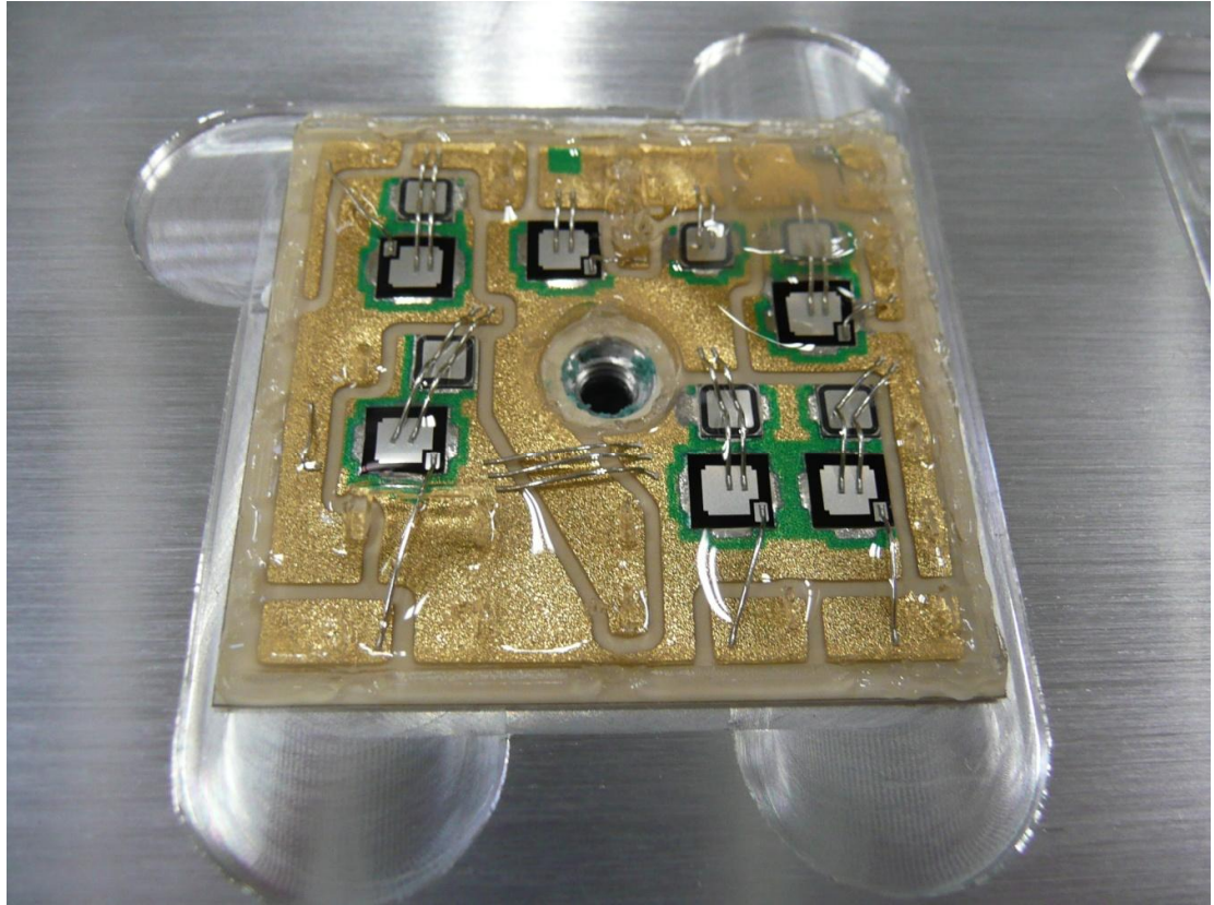
Figure 17: Bosch Rexroth's double-axis (2x 2,2 kW) inverter module IGBT which case came off during the disassembling.
