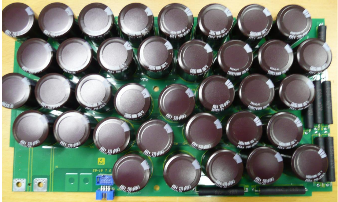
Figure 23: PCB of Bosch Rexroth's 2,1 mF capacitor bank
