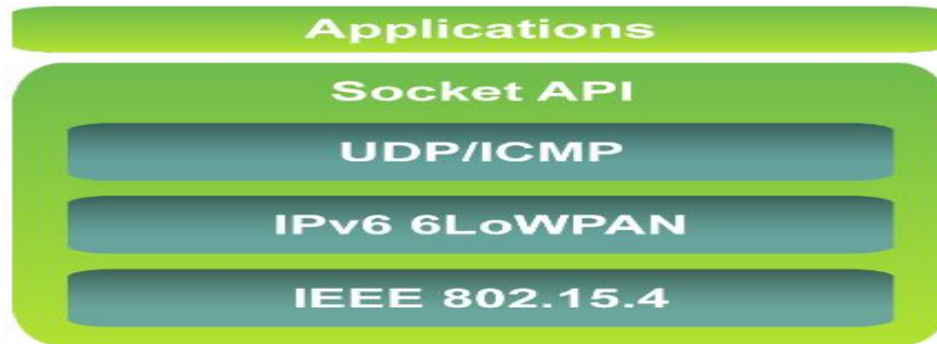
Figure 24: Architecture of NanoStck
