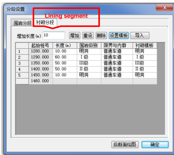
Figure 13. Lining segment settings by HintSD [21].
