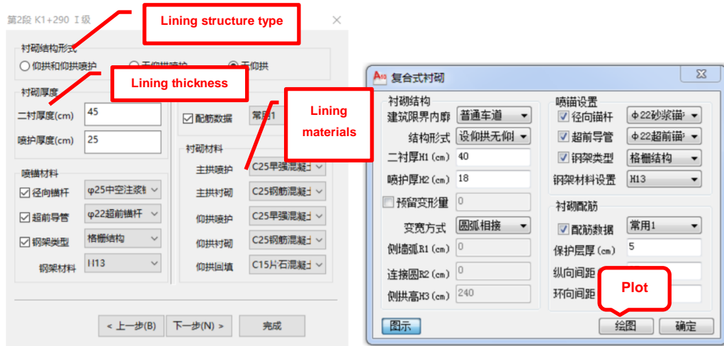
Figure 15. The lining structure design interface with HintSD. [21.]
