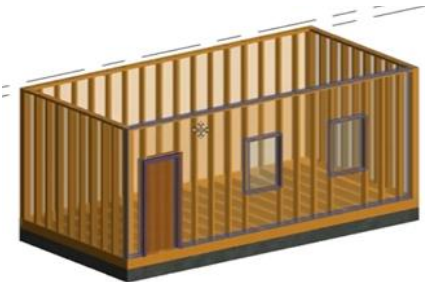
Figure 6.10 Arrangement of top plates
