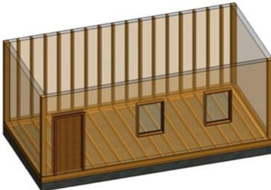
Figure 6.8 Arrangement of studs
