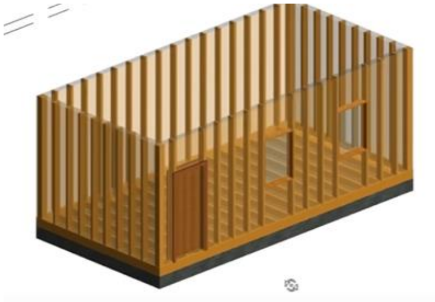
Figure 6.9 Completed arrangement of studs
