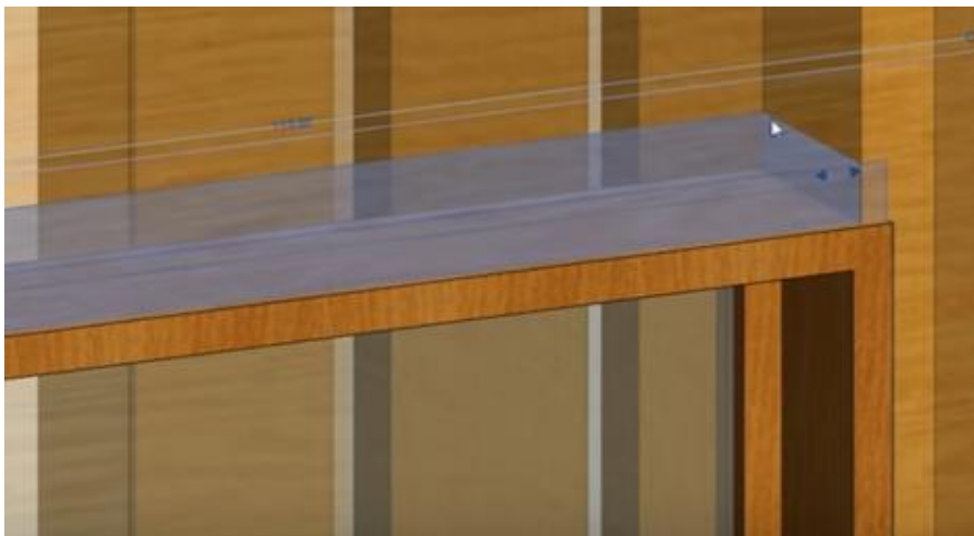
Figure 6.5 Detailed view of window bracing
