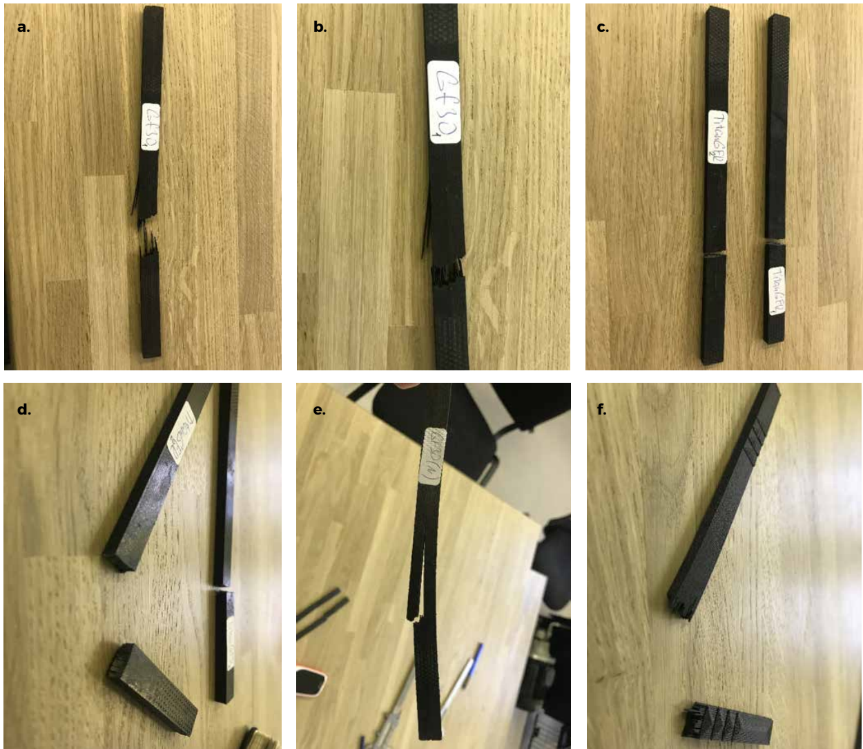
Figure 5. a. & b. Destroyed GF30 sample destruction of the material along the fibers. c. & d. Destroyed sample of Titan GF12 destruction of the material along the fibers; e. & f. Destroyed sample GF30 (N) destruction of the material along the fibers (Photos by Dmitrii Zhivotov)
