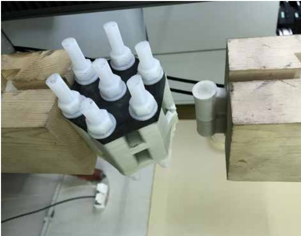
Figure 8. The destroyed joint (Photo by Dmitrii Zhivotov)
