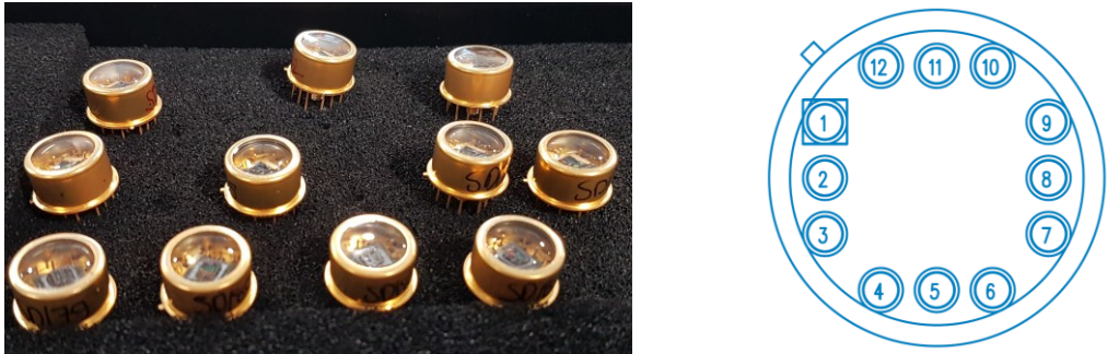
Figure 8. Emberion R&D photodetectors packaged in TO-8 cans which have 12 I/O pins.
