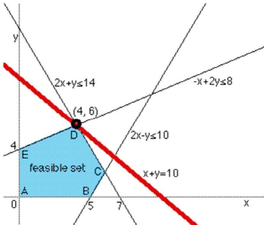
Figure 9. Graphical solution of a linear optimization problem
