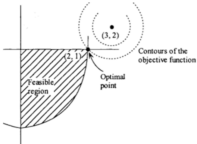
Figure 10. Graphical solution of a nonlinear optimization problem (Bazaraa et al. 2013, 3)
