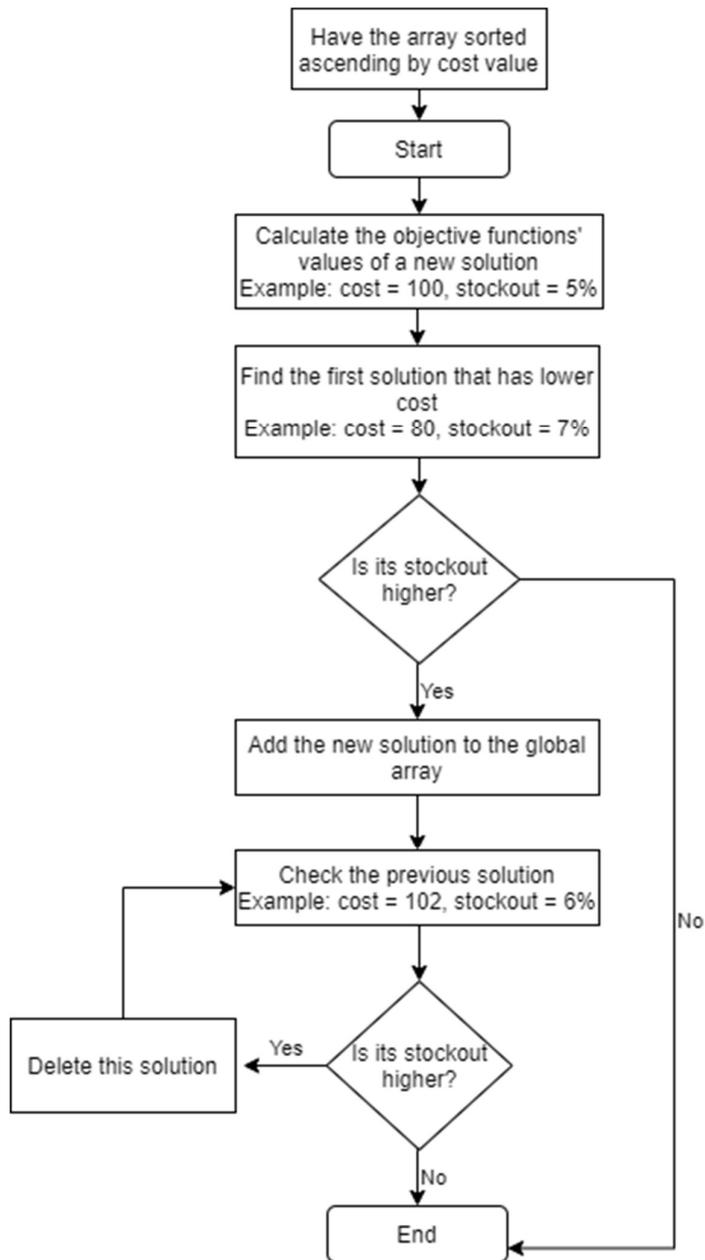
Figure 18. Optimality validation sub-algorithm
