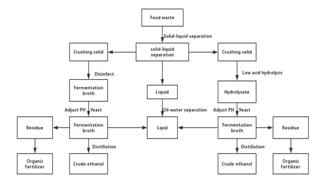
GRAPH 3. The process of preparation of ethanol from food waste. (adapted from Wang 2015)
