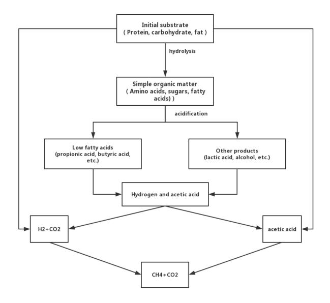
GRAPH 2. Three-stage diagram of fermentation. (adapted from Wang 2019)
