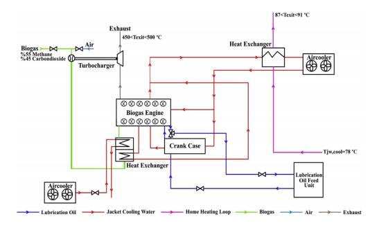
FIGURE 2. Engine schematic diagram. (adapted from Yağlı, et al. 2016, 923-932)
