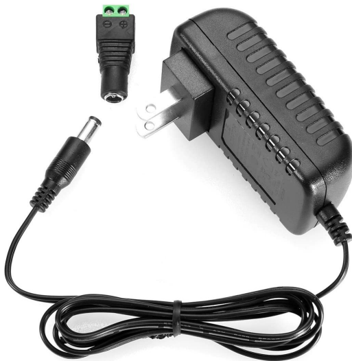
Figure 11. The power source for the system: 12V DC Power Plug Jack Adapter Connector and a 12V adapter (Amazon)
