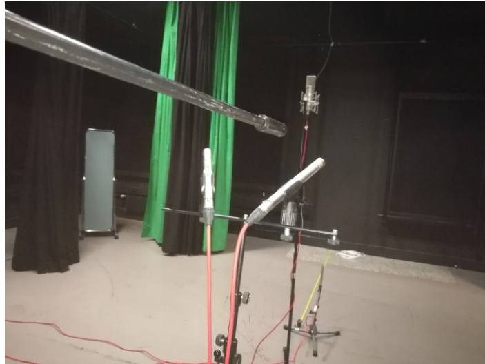
PICTURE 8. ORTF in the front, aimed to corners of the roof, with cardioid aimed to backwall and shotgun microphone aimed to roof (Hipponen, 2020).
