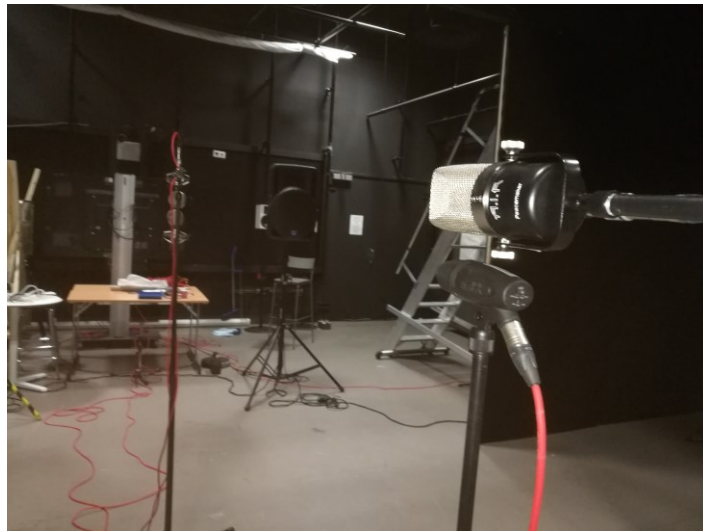
PICTURE 7. Mid-side and blumlein microphones with the right side of the PA. Small diagram condenser is placed under the table and a flat screen TV can be seen in the back. (Hipponen, 2020.)
