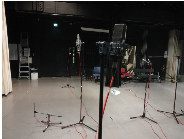
PICTURE 6. Right side of spaced omni pair, or A-B pair, at the close frame. Left side of A-B pair on the floor can be seen further in the image. (Hipponen, 2020.)
