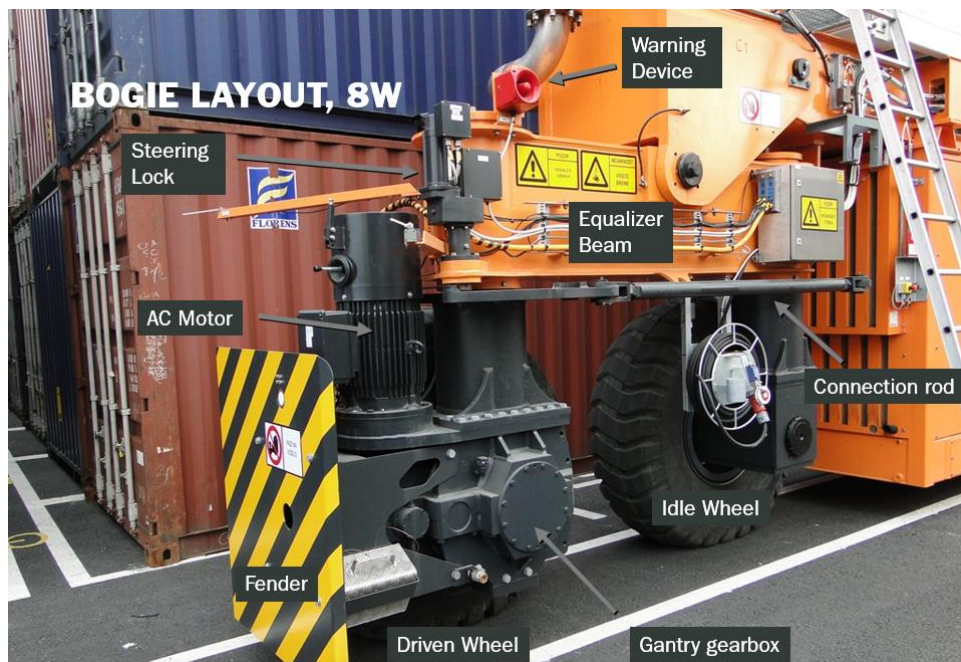
Figure 8 8-wheel Bogie layout (Rubber tired gantry cranes, 2012).
