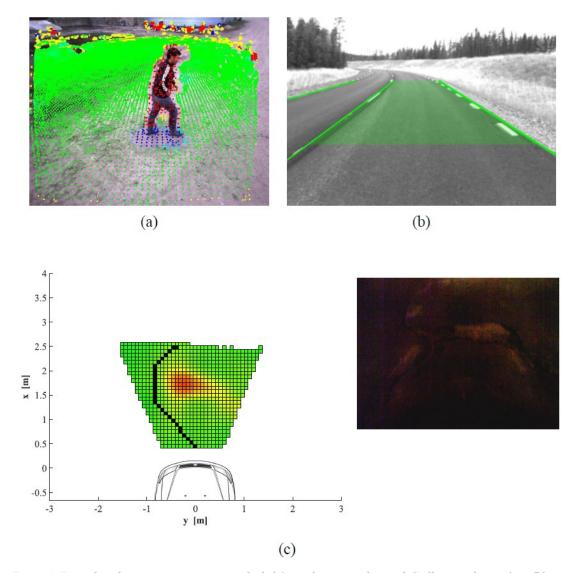
Figure 4: Examples of scene interpretation in which (a) a pedestrian is detected, (Bellone et al., 2013); in (b), the result of a lane detection algorithm is shown (Benderius et al., 2018); whereas in (c), an example camera vision mixed with depth inform.
