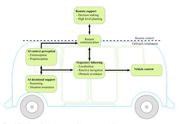
Figure 2: Main elements for situation awareness for an autonomous minibus
