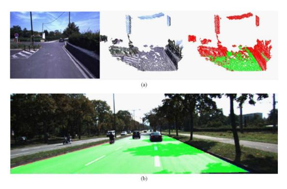
Figure 5: Road classification from 3D images using two different machine learning algorithms: (a) SVM classifier on 3D data, source: M. Bellone et al., 2017; and (b) deep learning approach on visual camera images enhanced with LiDAR information, source: Caltagirone et al., 2018.
