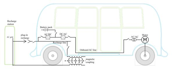
Figure 1: Electric components for a typical electric minibus
