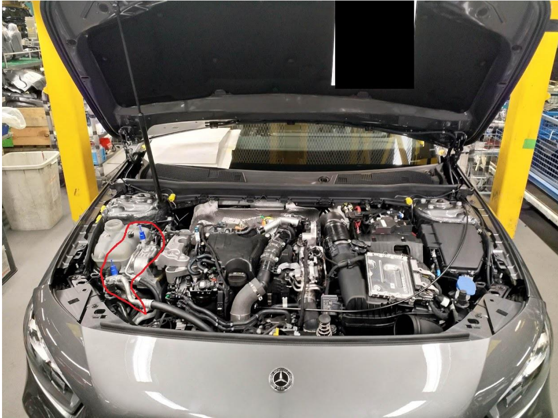
Picture 5 W177 engine compartment space. AC-pipes on the left side highlighted in red.
