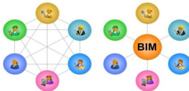
Figure 7: Conventional process versus the BIM process 14 .
