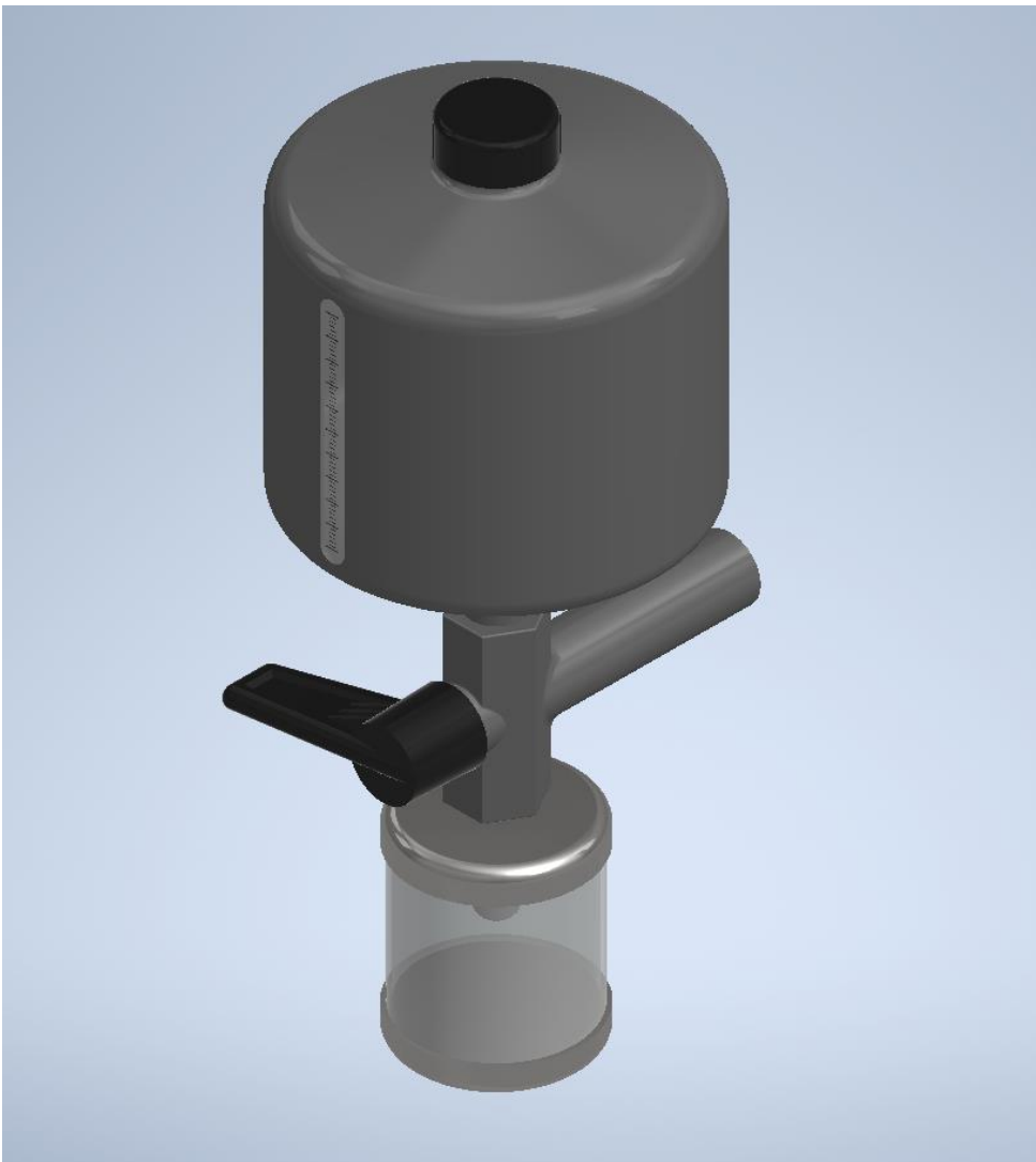
Figure 32. Water leak imitation device assembly
