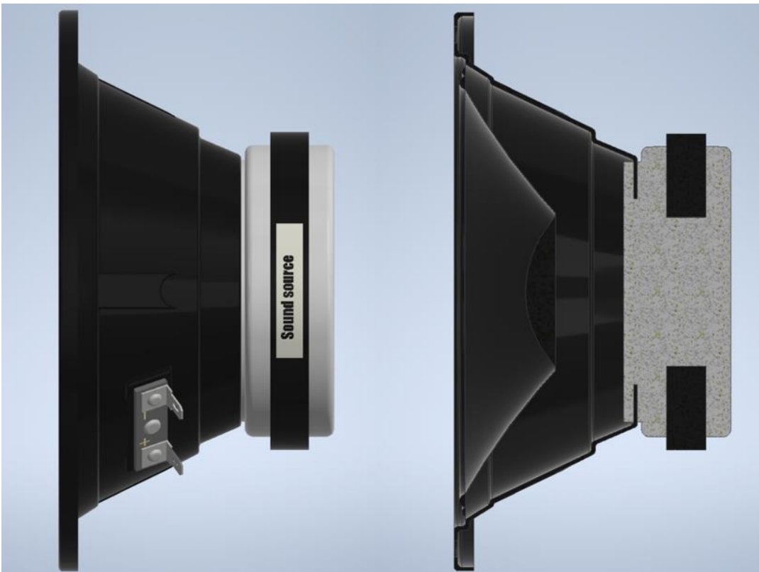
Figure 22. Sound source - side and cross-section view
