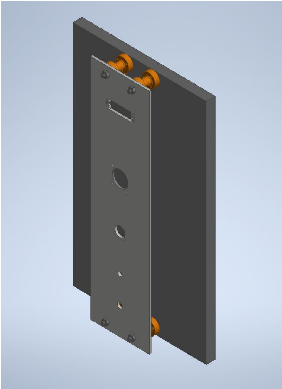
Figure 25. The plate for the electrical connectors
