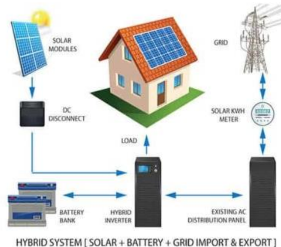
Figure 19. Hybrid PV configuration/ Apollo Power Systems [60].
