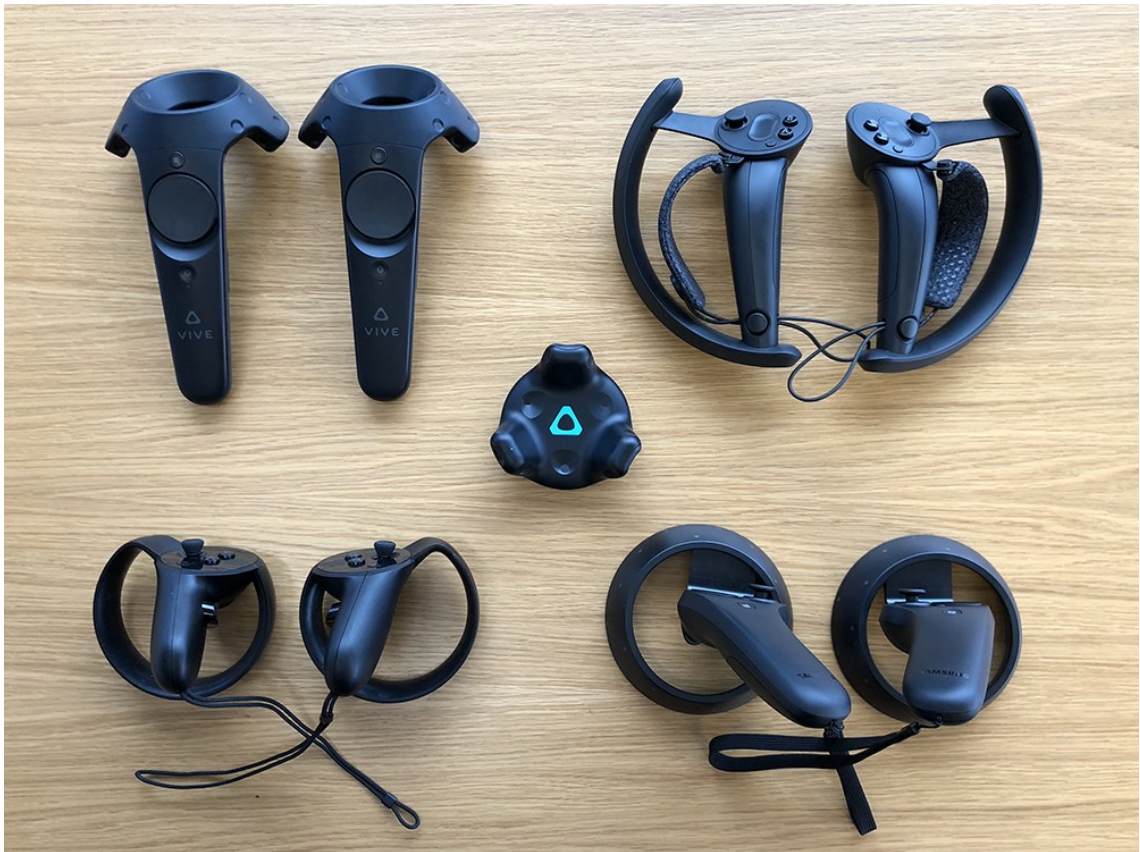
PICTURE 13. Different VR controller designs. Upper left: HTC Vive controllers, upper right: Valve Index's Knuckle controllers, lower left: Oculus Rift's Touch controllers, lower right: Samsung HMD Odyssey (WMR) motion controllers. (Steam 2018)
