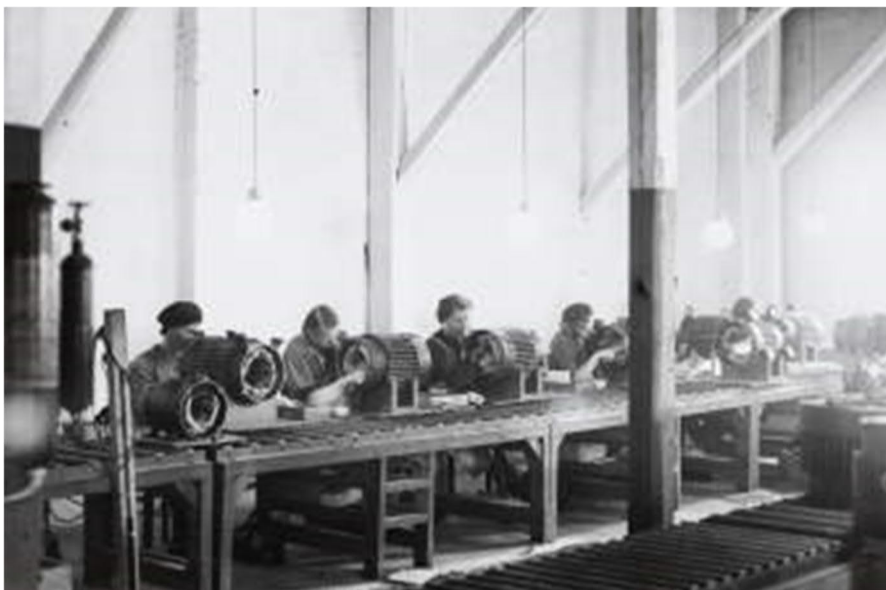
Figure 6. Motor stator winding line from 1943. (ABB history 2008)
